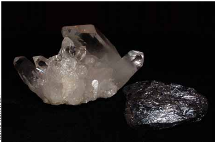
Figure 1: The transformation of quartz to silicon metal is the first step in making silicone compounds. Quartz is on the upper left, silicon on the bottom right.
