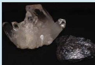
Figure 1. Silicone Compounds are ultimately derived from Quartz (upper left), which is converted into silicon metal (lower right). Picture © 2005 Thomas O'Lenick, used with permission
